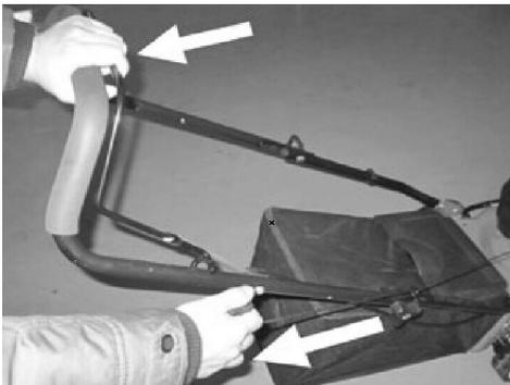
Blade is in action as soon as engine started. While the machine is working maintain the brake control handle in working position. The engine will stop as soon as you release the brake control handle.
