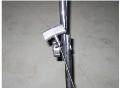
Introduce the rope of the recoil starter handle on its support rope guide.
