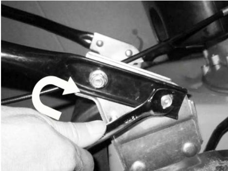
Fix the lower handlebars into the unit body with a suitable spanner.
