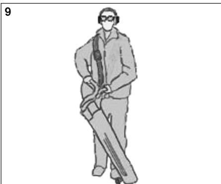
6. While standing in the operating position (Fig. 9) adjust the length to fit your height.
