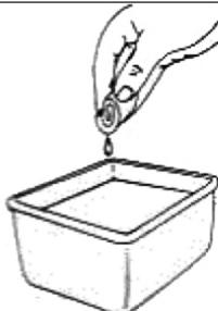
4. Apply enough clean oil to lightly coat the filter (Fig. 25).
