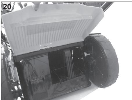
2. Press the lower side of the handle to release and remove the mulching insert (Fig. 20).
