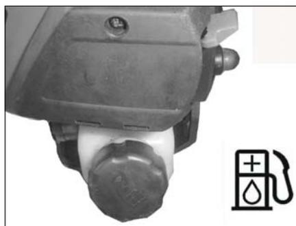
Before fueling, clean the filler cap and the area around it to ensure that no dirt falls into the tank.
