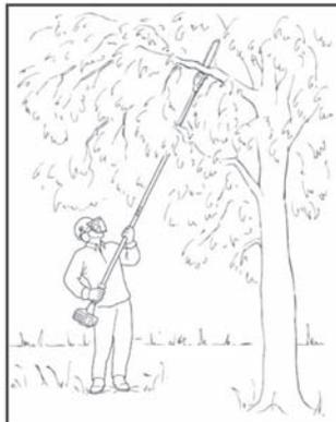
The shaft should always be held at an angle of 60° or less! The most convenient working position is a tool angle of 60°, but any lesser angle may be used to suit the situation concerned.
