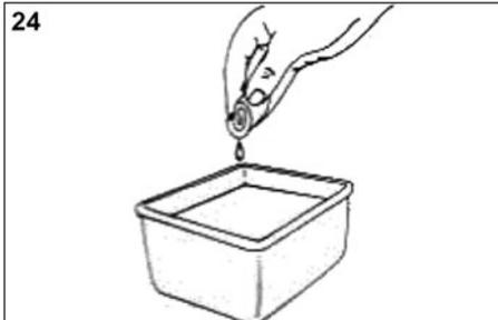
4. Apply enough clean oil to lightly coat the filter (Fig. 25).
