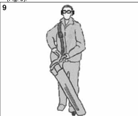
6. While standing in the operating position (Fig. 9) adjust the length to fit your height.
