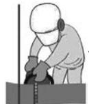
11. Keep all parts of your body away from the saw chain when the engine is running. Before you start the engine, make sure the saw chain is not contacting anything.
