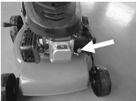
When starting a new engine for the first time, firmly push the yellow primer five times. Then for all future starts, push the primer three times.
