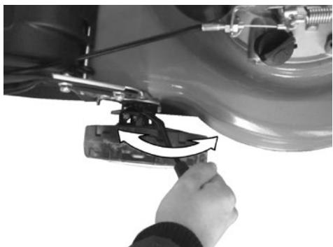
Apply outward pressure to disengage lever from rack, move lever forward or back to adjust height.
