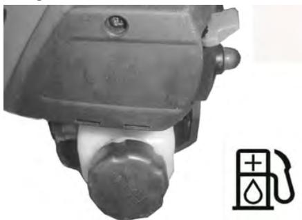
Before fueling, clean the filler cap and the area around it to ensure that no dirt falls into the tank.
