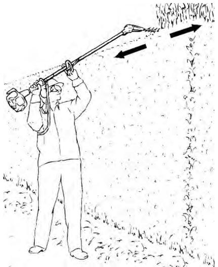
Any working position above head height is tiring. To minimize the risk of accidents, work in such positions for short periods only. Set angle of adjustable cutter bar to maximum so that the unit can be held in a lower, less tiring position (with harness) while still providing adequate vertical reach.
