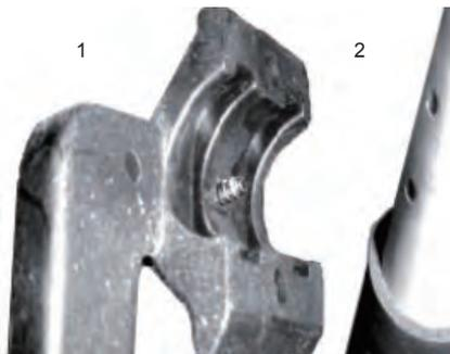
Position the screw (1) into the hole of the driver tube (2). Note there have four holes follow your request.
