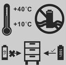
Charge between +10°C and 40°C. Keep the battery away from water and moisture. Charge rechargeable battery before storing.
