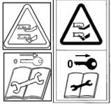
Warning! Sharp blade! Remain at a safe distance from the moving blade when operating.
